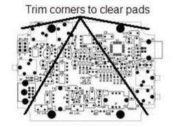
Using a Dremel® tool with a sanding drum or a round file, remove the rough edges from the corners. Be sure the board will fit inside the top enclosure without interference from the molded screw posts before proceeding.
